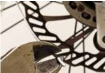
Cutting the cable end
