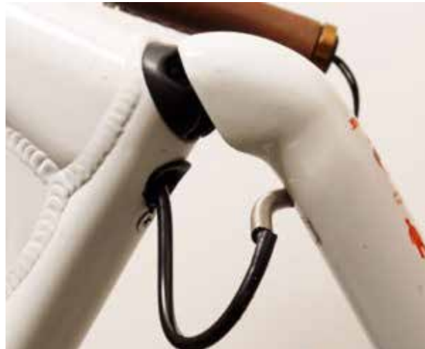
Removing the cable housing
